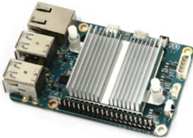
Heatsink applied to ODROID-C1
